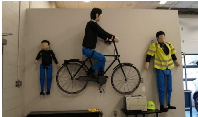
Surrogate pedestrian and bicyclist testing devices for high-risk crash scenarios
