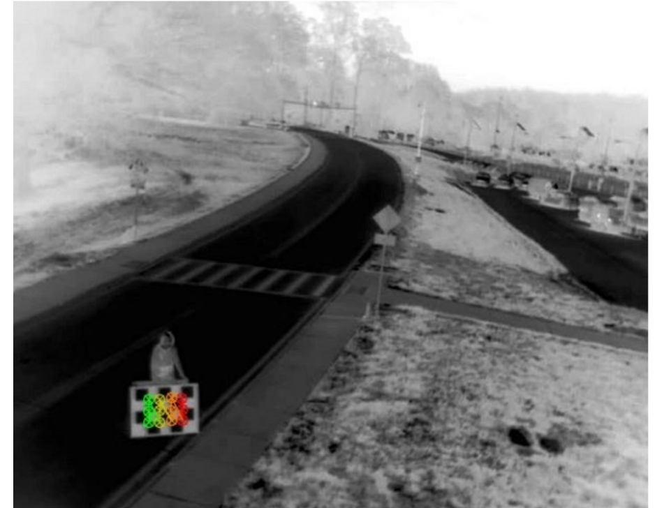
Thermal image enhancement example for visual camera-thermal camera pairwise extrinsic calibration.
