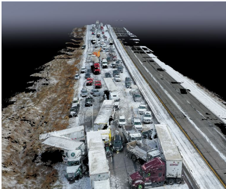
Figure 13. Unmanned Aerial System 3-D Imaging Used for Crash Investigation Source: Iowa State Patrol.
