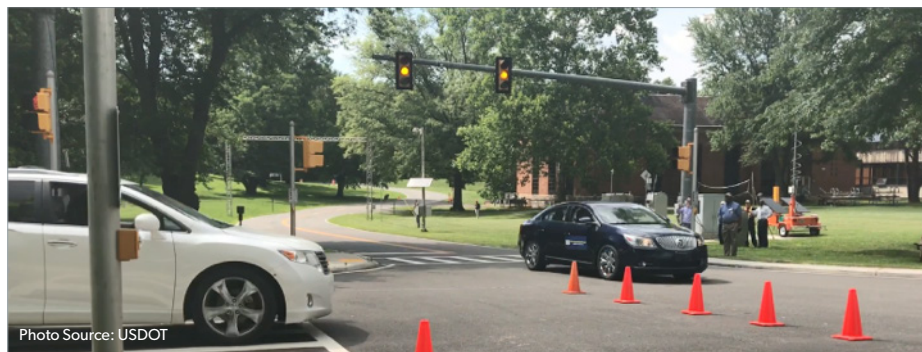
A Tampa vehicle receives an intersection movement assist warning being triggered by a New York City vehicle
