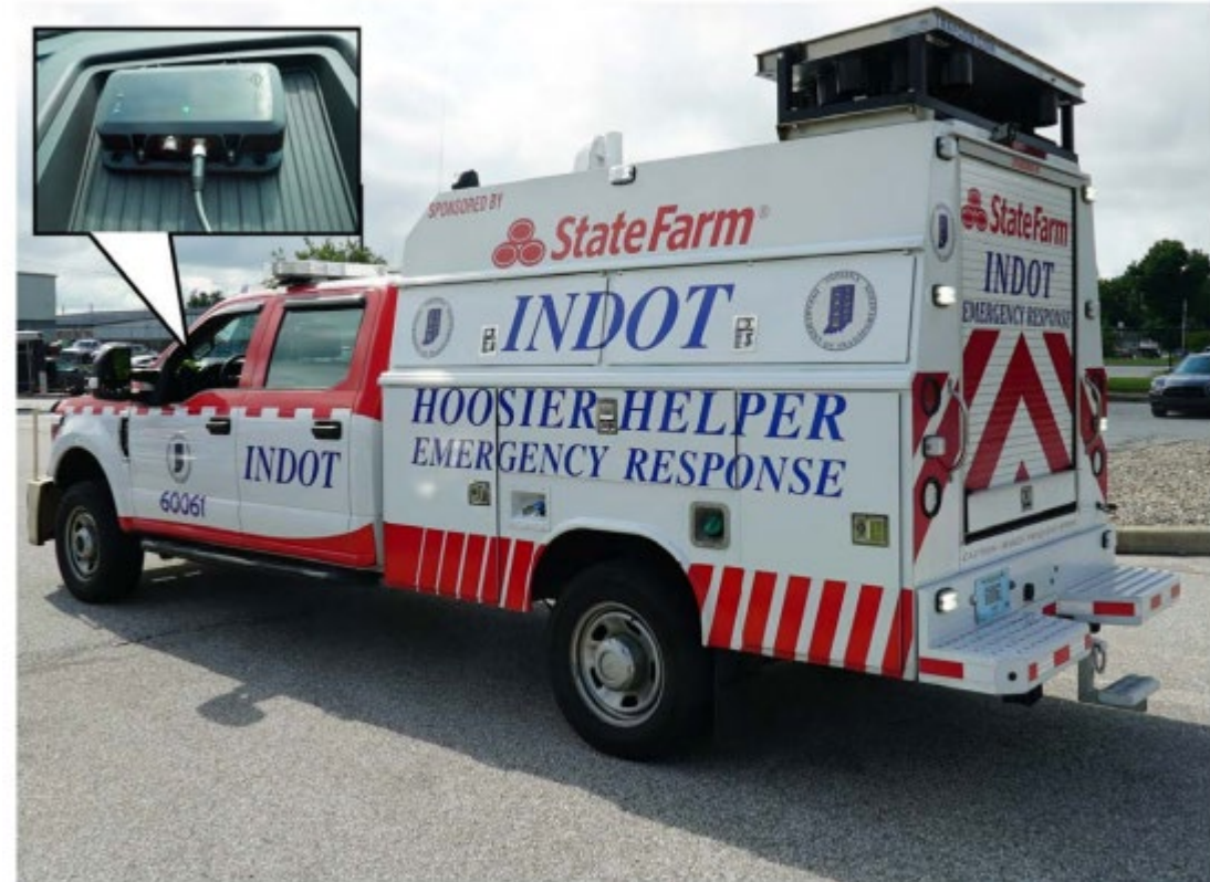
Hoosier Helper emergency response vehicle equipped with onboard transponder. Source: Indiana DOT
